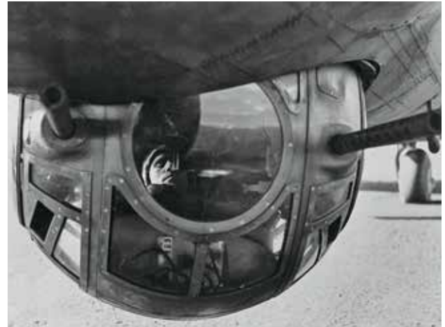
↑ A gunner tests the equipment in the ball turret, which was one of the most cramped, and dangerous, spots for airmen in the B-17.
