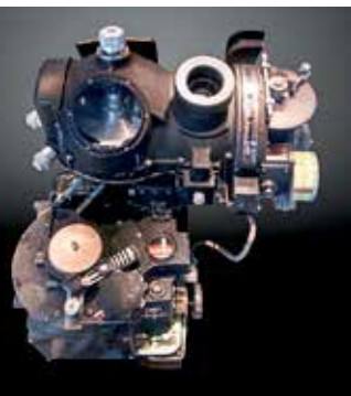
The new Norden bombsight improved accuracy of high-altitude bombing.
