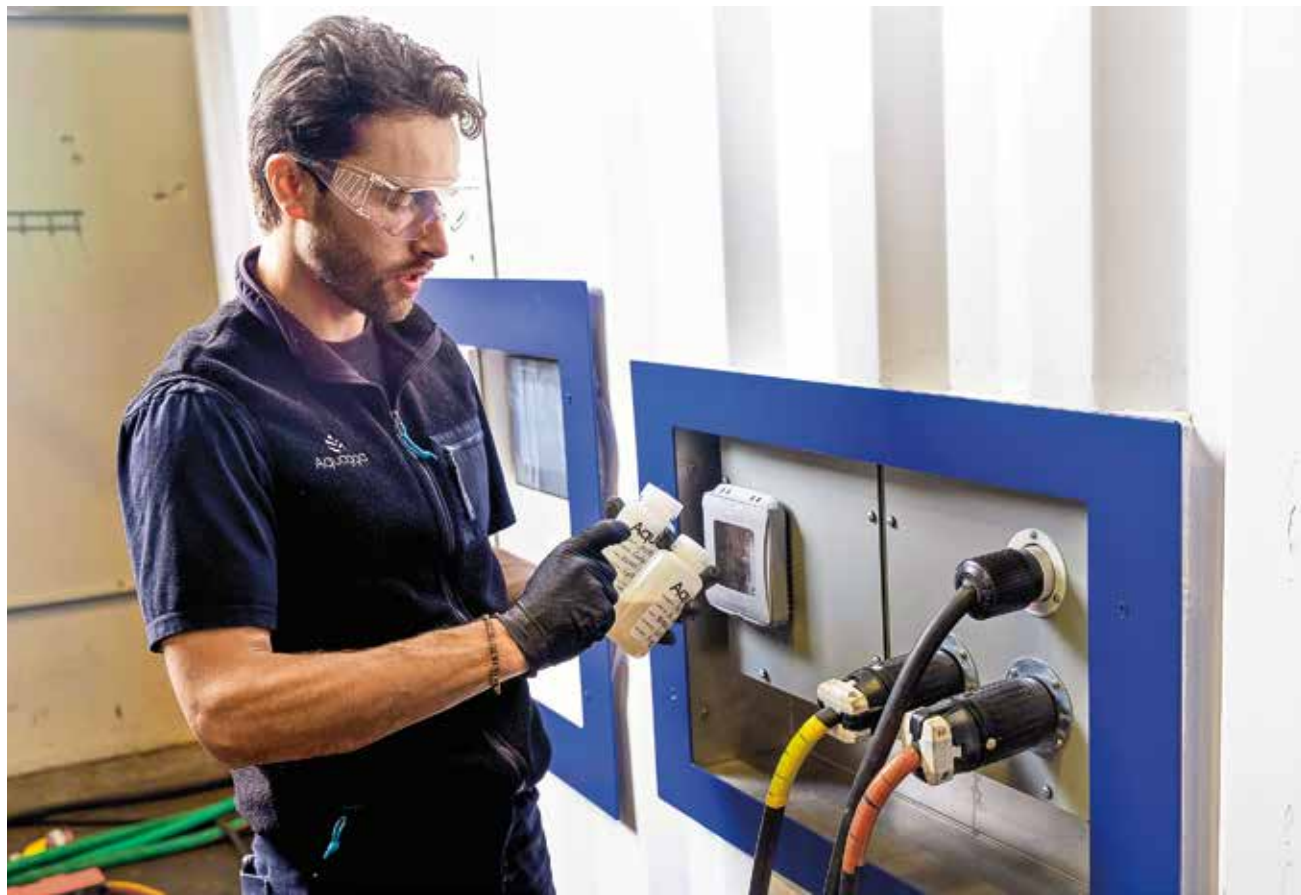
Aquagga’s hydrothermal alkaline treatment technology, which won the EPA’s Destroy PFAS Challenge in 2022, uses chemicals and hot compressed water to help break apart the strong carbon-fluorine bonds. Mobile units like the Steed Series, pictured here, can treat 10 to 100 gallons per hour.
